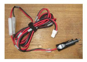
The vehicle radios do not need any kind of "installation" in the vehicle – the power lead just plugs in to the 12 volt "cigarette lighter" socket found on most cars, vans etc, and the magnetic aerial will attach to the roof of any steel-bodied vehicle.
